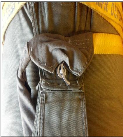
Main Curve Pin of an T-11 ATPS with the pin in the improper position.
