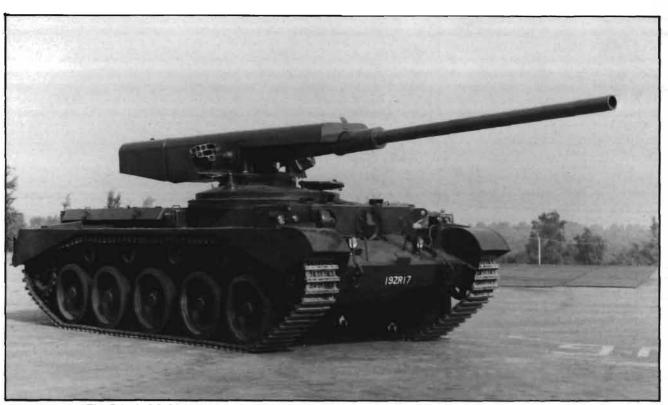
The British COMRES 75 test bed vehicle was built in 1968 to explore externally-mounted main guns.
