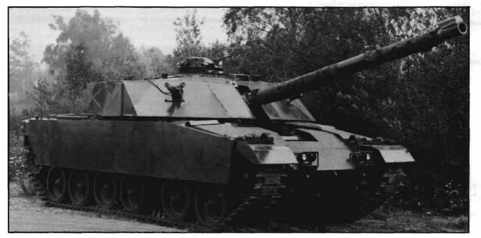
The British FV 4211, first test bed vehicle to incorporate Chobham armor.
