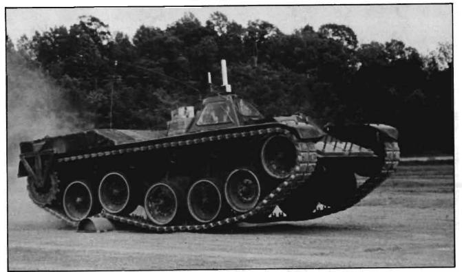
The U.S. HIMAG test bed was used to study various mobility and fire control options.
