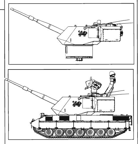
The Navy 76/62 deck gun, with autoloader, is available as a turret unit that can be installed, with its turret basket, in an MBT chassis.
