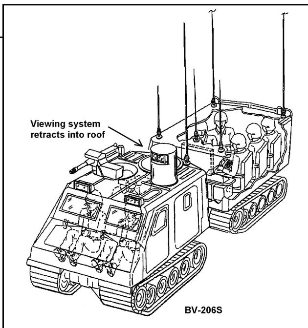
Proposed battle command variant of the BV-206S, an armored version of the Army's M973A1. Schematic of command and control architecture is seen below.
