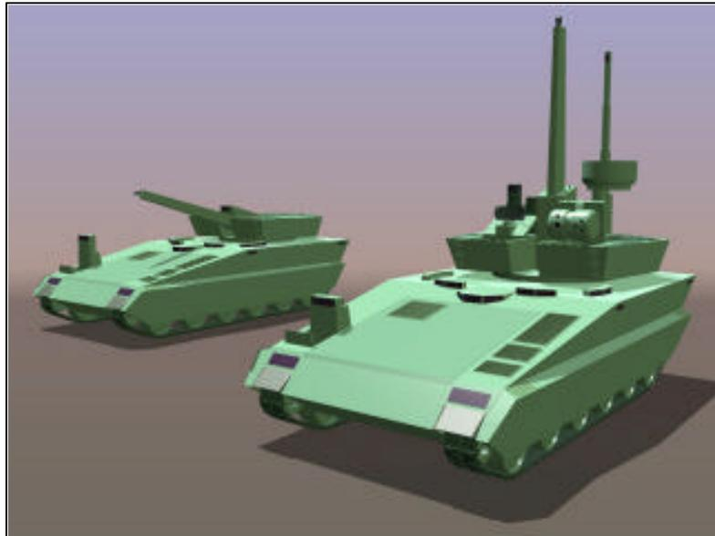
emy. Stringent operational requirements have been posted for a small and light vehicle featuring a low profile, increased agility, and improved mobility to enhance its survivability. These requirements led to various vehicle configurations that were inadequately protected — if at all — thereby suffering a highly disproportional casualty rate when exposed to hostile enemy fire.
