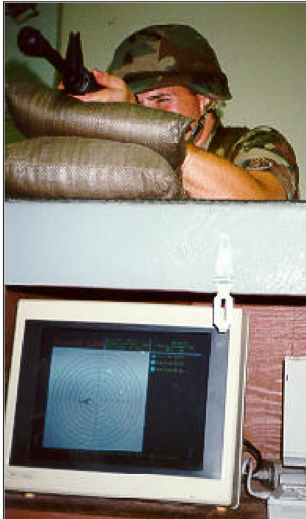
The results of SGT Megow's three-round shot group. The darker circle on the monitor indicates the center of mass of the three-round group. The results are within the 40mm dispersal required.
