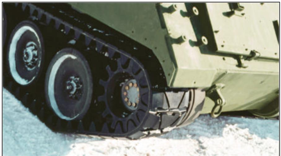
Detail view of the continuous band track installed on an M113 APC during recent tests.
