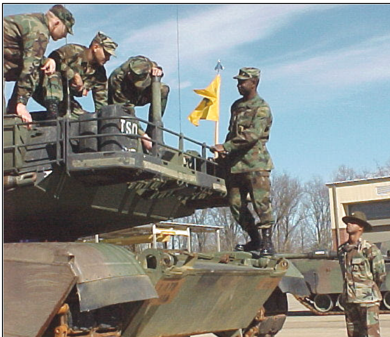
Drill Sergeant Dennis Bellinger observes as the Tank Commander, SFC Willie Hicks , trains soldiers on how to erect the crosswind sensor of D15.
