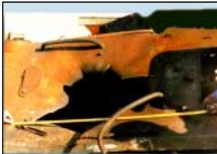
Effects of the BDM against concrete block wall (left), and BMP armored personnel carrier (right)
