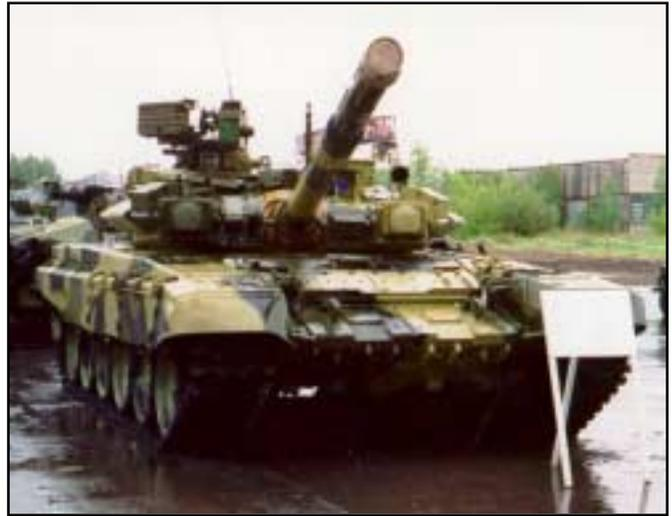
T-80, left, and T-90 on static display, painted with an electromagnetic wave deforming/absorbing coating to prevent radar detection.
