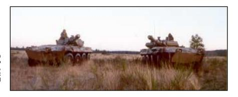
While the U.S. version of the Medium Gun System is being re-engineered to reduce its height for C-130 deployment, troops of the Interim Brigade Combat Teams are training on Centauro armored cars borrowed from the Italian Army.
