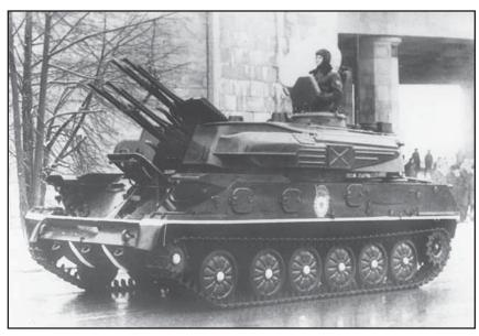
"The Russians discovered that the thinly armored ZSU 23-4 self-propelled antiaircraft gun was the optimum system for tank support in city fighting, but its vulnerability offset the efficiency of its four 23mm automatic cannons. To ensure the survivability of tanks, they needed a new system that was built like a tank, but provided mutual close combat support."
