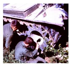
Figure 13, above. Repairing a track thrown to the inside of the sprocket when navigating a narrow path in Germany in 1965. No fun, as the other track was thrown, too.
