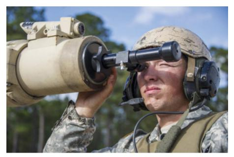
Figure 2. SPC Cody Winder, an M1A2 System-Enhancement Program Abrams loader for 2<sup>nd</sup> ABCT, 3<sup>rd</sup> Infantry Division, conducts bore-sighting procedures during live-fire accuracy screening. (*Photo by SGT Richard Wrigley*)
