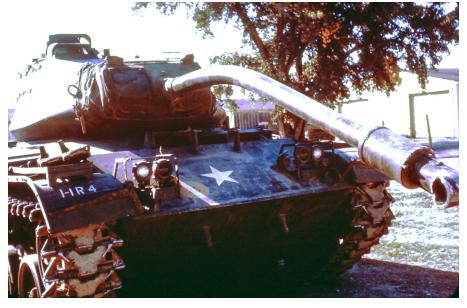
Figure 2. A 1<sup>st</sup> Battalion, 4<sup>th</sup> Cavalry (1<sup>st</sup> Infantry Division), M41 tank at Fort Riley, KS, in September 1963. The photographer's tank ran over its own gun tube when crossing a steep stream bank at night.
