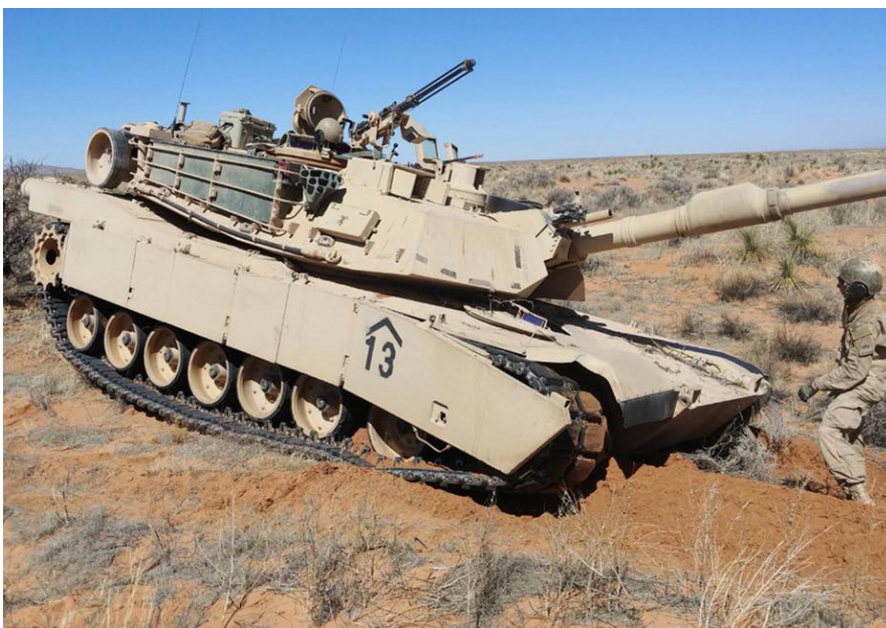
Figure 2. Red Platoon conducts recovery operations since the platoon leader’s tank threw a track. (U.S. Army photo by 1LT Justin Leugers)
