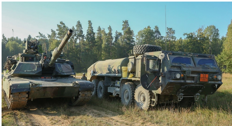
Figure 1. A Heavy Expanded-Mobility Tactical Truck fueler prepares to conduct refuel operations in an austere environment. (U.S. Army photo)
