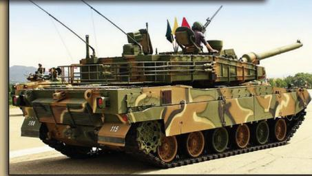
South Korean main battle tank, first fielded in 2014. Three-man crew, 55 tons weight. Autoloading 120mm L/55 main gun, with fire-and-forget capability. Advanced ERA and NERA armor protection. Advanced fire control and radar warning system. In service with: Republic of Korea Army.
