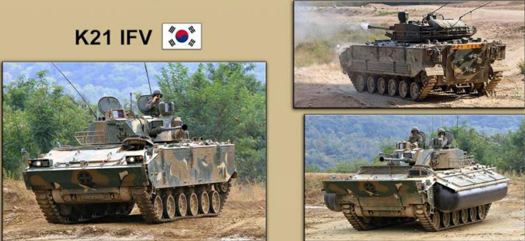
South Korean infantry fighting vehicle, first fielded in 2009. Three-man crew plus nine passengers, weight 25.6 tons. Main armament is a 40mm autocannon, 7.62mm main gun secondary. Layered fiber-reinforced ceramic modular armor and advanced fire-control / stabilization system, which allows accurate shoot-on-the-move capability. In service with: Republic of Korea (RoK) armed forces, with 400 vehicles produced to date.
