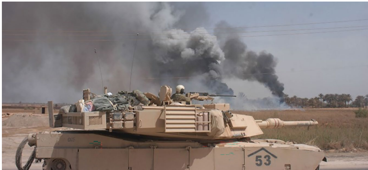
Figure 9. An M1A1 of the 3 rd Infantry Division during Operation Iraqi Freedom I. The extended bustle rack was fabricated before the invasion began when it became clear that division combat units would need more supplies than their trains could accommodate. (U.S. Army Armor School Branch Archives)
