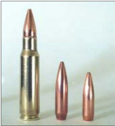
*The 6.8x43mm special purpose cartridge (left) was developed to provide special operations forces increased incapacitation potential in close combat. However, to make a round that is better suited for general purpose use, the SPC case should be necked down and loaded with a more ballistically-efficient 6.5mm (center) or 6mm bullet (right).*
