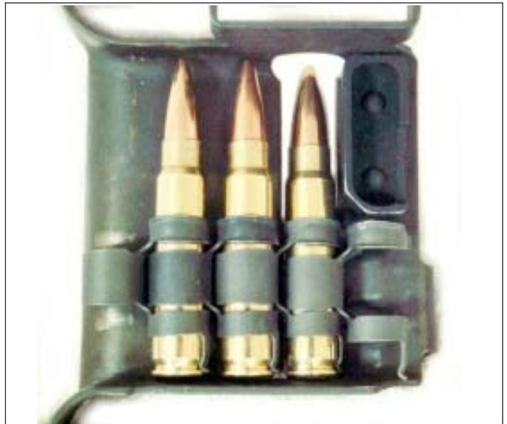
**Figure 6** — The 6x45mm (not shown) and the 6.5mm MPC, seen here plugged into standard M27 links and positioned on an M249 feed tray, essentially require only a barrel change for conversion of the LMG. However, the 6.8mm SPC and 6.5mm Grendel, need a new series of links designed and manufactured, and the M249 feed mechanism modified.
