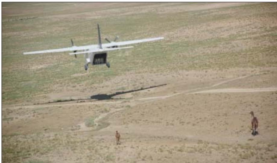
*Due to low altitude of the aerial delivery platform, the resupply bundle descends to the drop zone within seconds; this short descent time limits the ability of the enemy to observe the bundle.*
