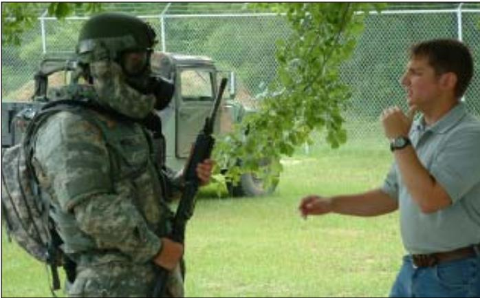
*Above and at right, the second demonstration evaluated eight face protection candidates and six neck protection candidates. Devices that offered the highest protection coverage received the lowest acceptance ratings from Soldiers because of the negative impact on mobility.*
