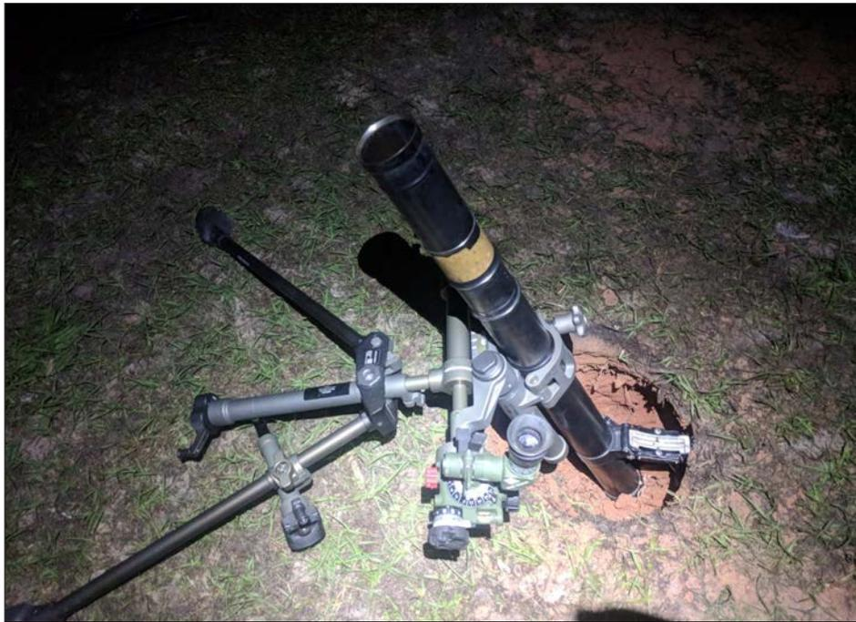
**A 60mm mortar base plate digs into the ground due to poor soil conditions.**
