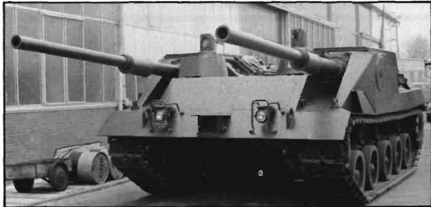
loader, it is possible to design tanks which are very different from those of the past 50 years. In particular, it is now possible to have tanks with guns which are not only automatically loaded but also remotely controlled and, therefore, mounted externally on pedestals or in small-frontal-area, unmanned turrets. The advantages in either case include much smaller exposed areas in defilade positions, reduced internal volume and complete separation of ammunition from the crew.
