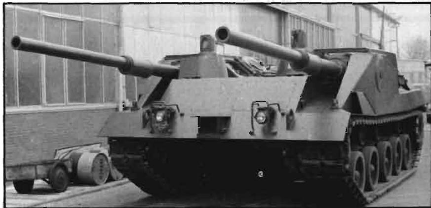
loader, it is possible to design tanks which are very different from those of the past 50 years. In particular, it is now possible to have tanks with guns which are not only automatically loaded but also remotely controlled and, therefore, mounted externally on pedestals or in small-frontal-area, unmanned turrets. The advantages in either case include much smaller exposed areas in defilade positions, reduced internal volume and complete separation of ammunition from the crew.
