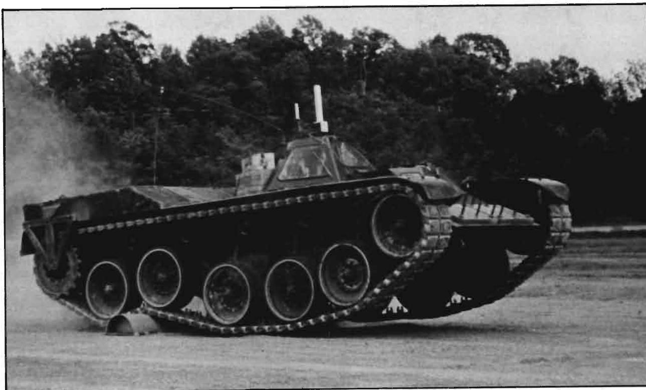
The U.S. HIMAG test bed was used to study various mobility and fire control options.
