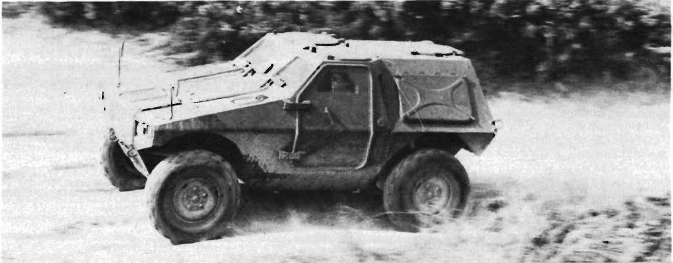
The M11's militarized Peugeot diesel, developing 105 horsepower, gives the vehicle a top road speed of 60 MPH. Above, the prototype demonstrates its high-speed cross-country performance. At right, the M11 is shown with an armament package that includes the Milan anti-tank missile and 7.62-mm machine-gun.
