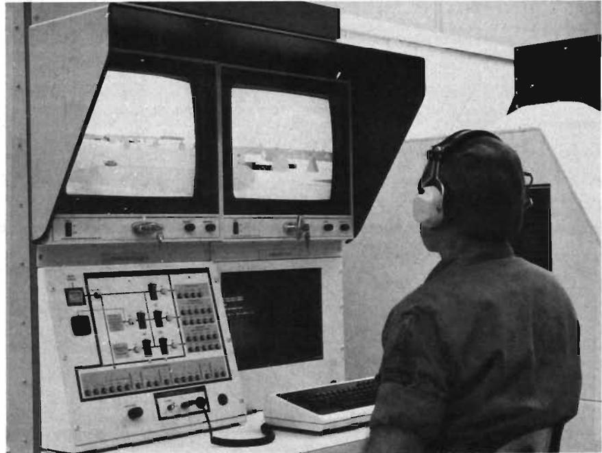
A technician at the evaluator's station sees both commander's and gunner's views on TV monitors. View on right hand screen is a magnified section of same view on screen at left.
