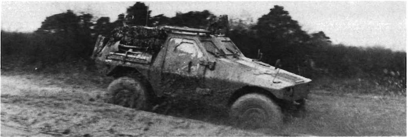
The M11's low ground pressure of 11 lbs. per square inch enables it to move over soft ground with ease. Reduction gears at each wheel have the effect of increasing ground clearance without adding additional height to the vehicle.
