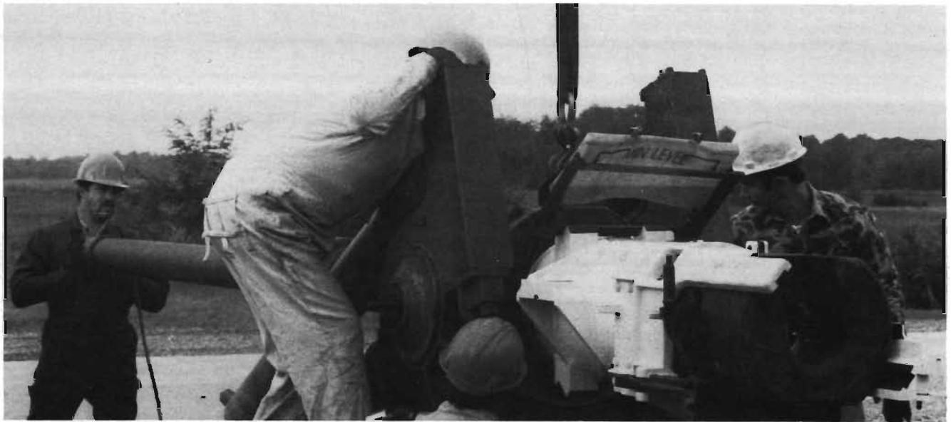
**Aberdeen technicians mount a 105-mm gun on a test rig prior to proof firing. Elaborate measurements taken**
