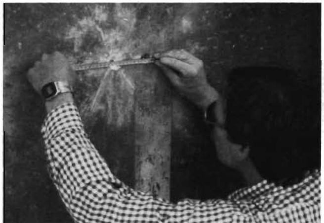
An Aberdeen technician measures penetration and diameter of a hit on armor plate made by an AT4 rocket from the new antiarmor weapon now under test at the Proving Ground in Maryland. The AT4 is said to penetrate 450-mm of armor.
