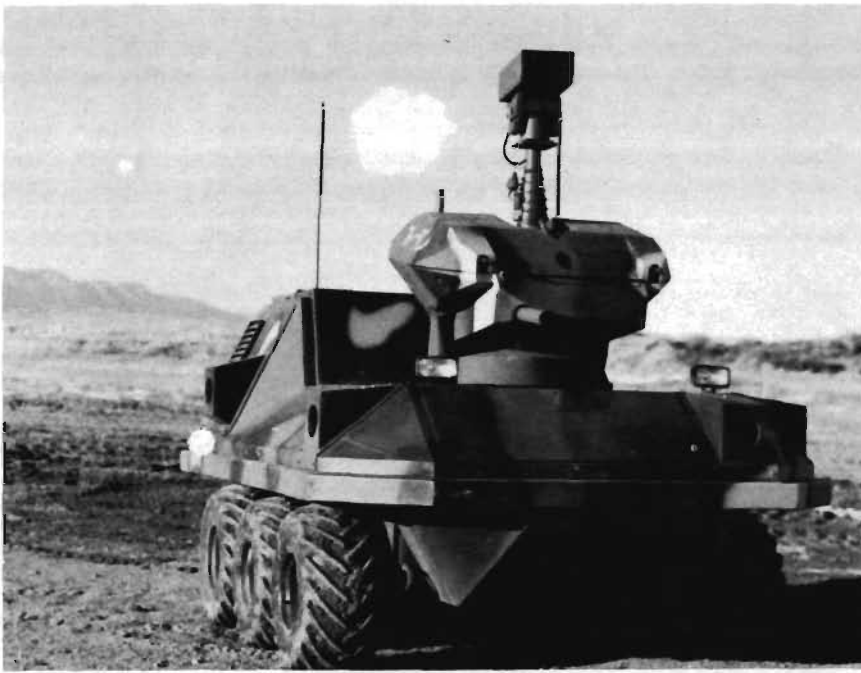
The 6-wheel, all-terrain PROWLER can sense motion, follow orders, and send back television views of a remote scene. The operator can also communicate over an audio channel.
