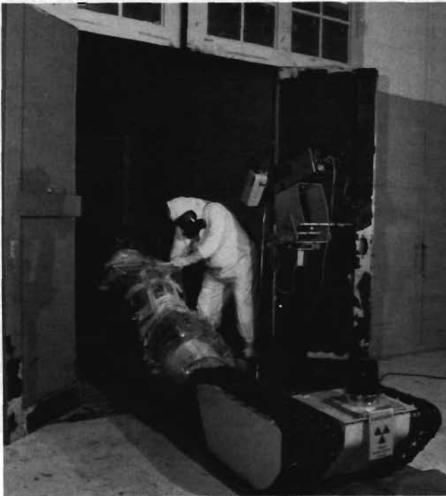
Radio-controlled, with television feedback, the 250-pound ROCOMP, at left, is seen here moving radioactive material in a test at Battelle Corporation. The autonomous land vehicle (ALV), seen at right as an artist's conception, is a Martin-Marietta Aerospace project.
