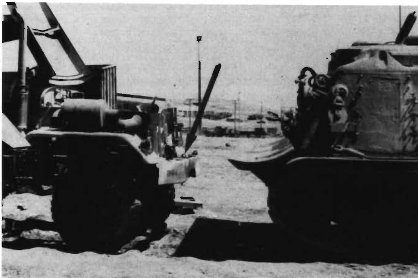
A ground guide attempting to position this M88 recovery vehicle in a salvage operation was crushed between the M88 blade and the truck at left when the M88 shift lever malfunctioned and the vehicle moved in the wrong direction.
