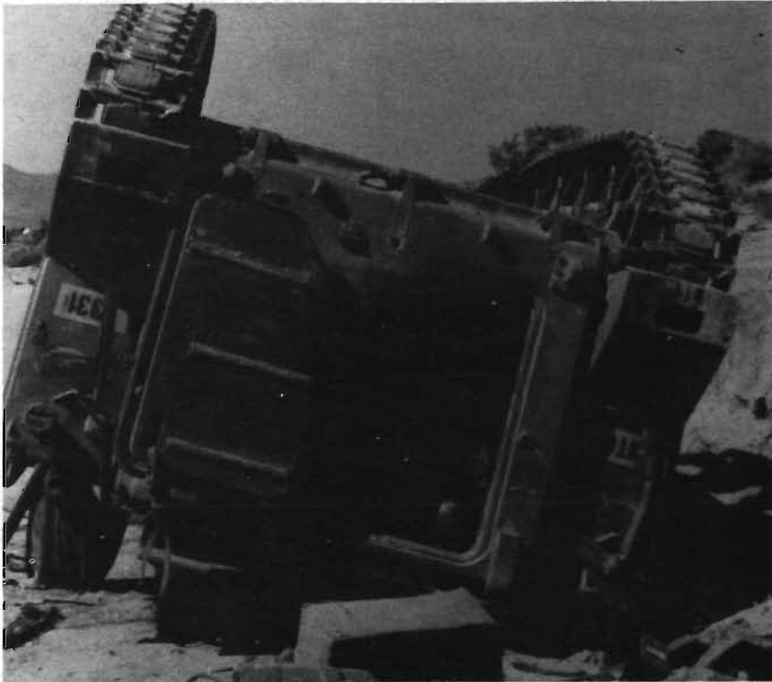
An observer in the crew hatch of this M113 was killed when the vehicle overturned on a washed-out tank trail. The cargo in the carrier shifted as the vehicle overturned, pinning the soldier and ultimately suffocating him.
