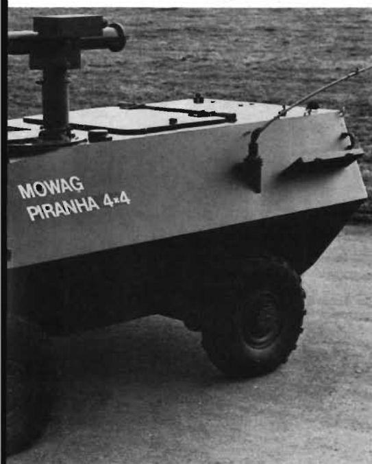
Piranha 4 x 4, above, and the Marines LAV-25, an amphibious fighting vehicle, at right, bear a strong family resemblance. They were developed from the same basic chassis.
