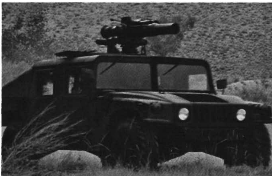
The High-Mobility Multipurpose Wheeled Vehicle (HMMWV), seen above with a TOW system mounted, has a big role in the new light infantry divisions. Other U.S. projects include the FAST-V, at right, and the LAV-25, below, the Marines' Light Armored Vehicle (LAV), which is much heavier (14.1 tons) than an ultralight, but easily transportable by air.
