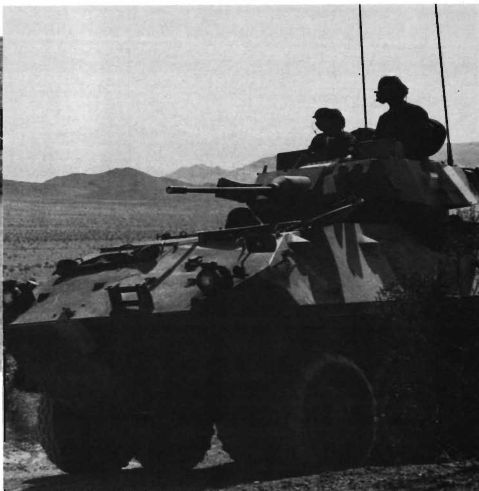
Piranha 4 x 4, above, and the Marines LAV-25, an amphibious fighting vehicle, at right, bear a strong family resemblance. They were developed from the same basic chassis.
