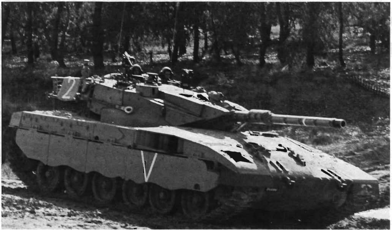
With turret set back on front-engined hull, Merkava has little gun tube overhang.
