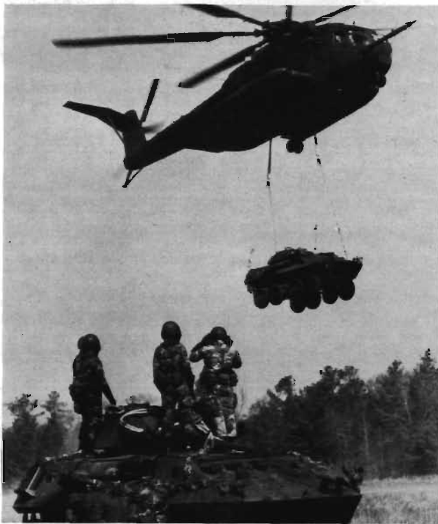
Shown above a Marine Corps H-53E helicopter prepares to land a 12-ton LAV 25 armored fighting vehicle during a tactical exercise that tested the new concept of two-point sling loading and the feasibility of the new airmobility tactic.
