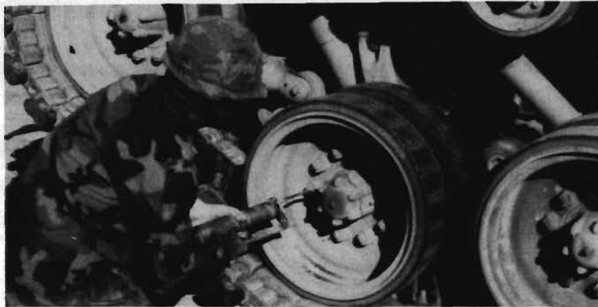
The Guardsmen's relatively trouble-free road march hinged on aggressive preventive maintenance. Here, road wheel bearings get a shot of grease during scheduled halt.
