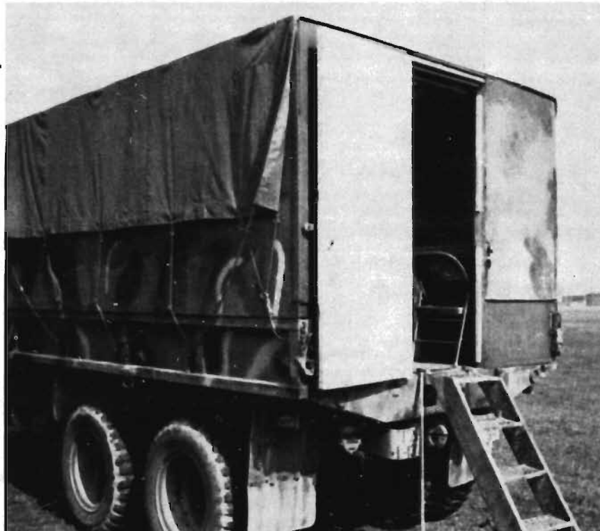
Photo 5. A 2½-ton truck, configured as a sleeping van, can accommodate six men off-duty. The truck eliminates need to set up tents and can redeploy fast.
