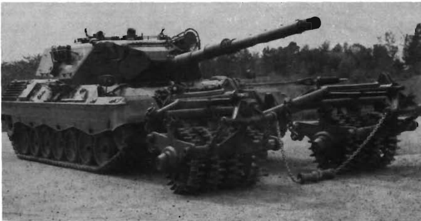
Figure 3. A Canadian tank-mounted mine roller.
