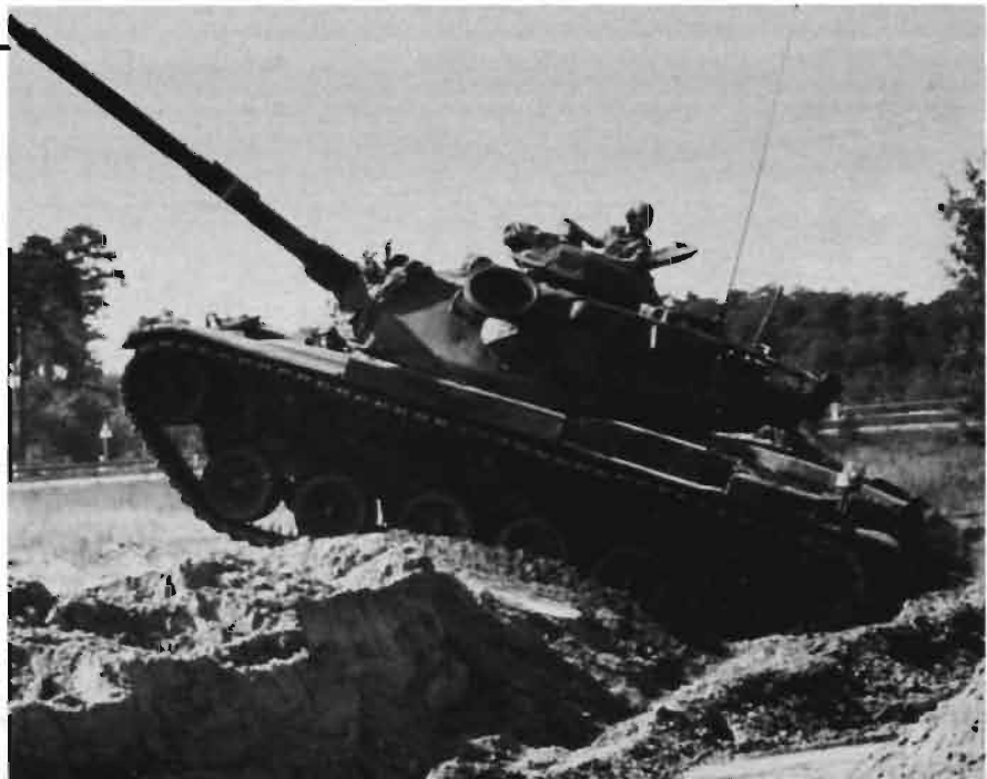
Extent of tank's vulnerability to a belly shot is apparent in this photo of test M60A3 climbing the berm. The advantage would increase if friendly forces were level with or below level of the berm.
