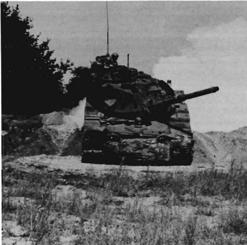
Tank bump also exposes a tank's thinner top armor to killing shots as it descends the berm.
