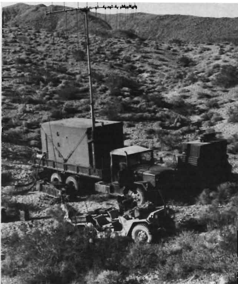
Truck-mounted XM-330 jammer and jeep-mounted direction finder, with azimuth indicator and receiver on rear fender, used by OPFOR at the NTC.
