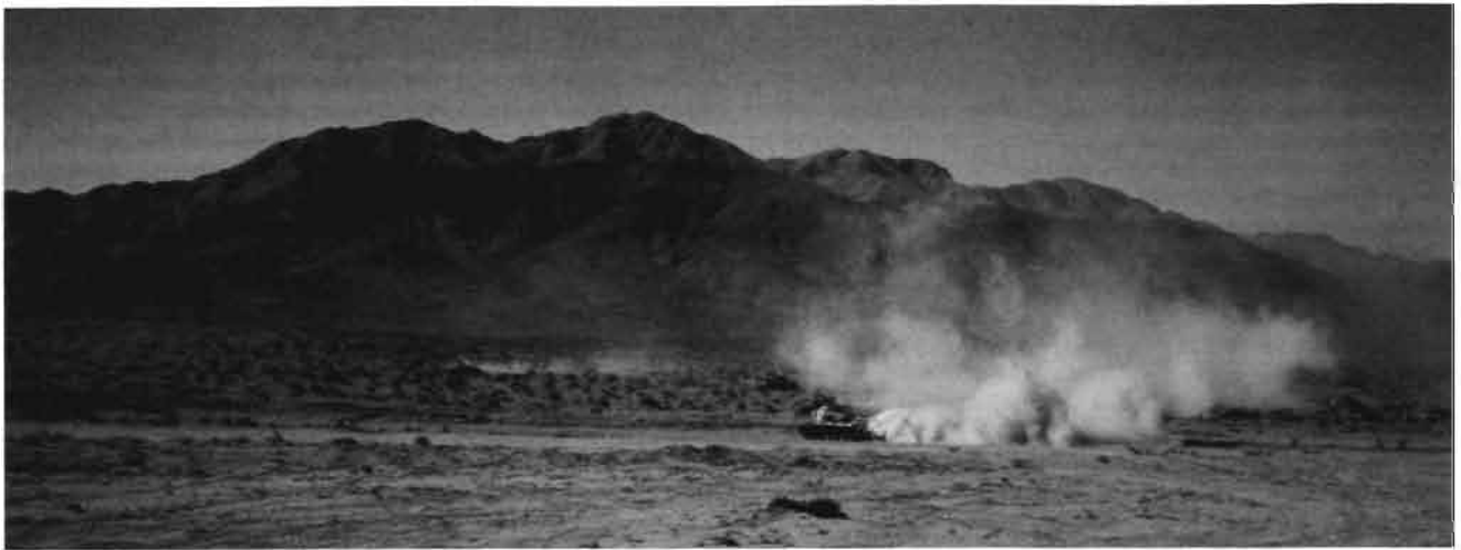
The most effective use of on-board smoke generation is during actual contact. Indiscriminate use of smoke can compromise a vehicle's position.
