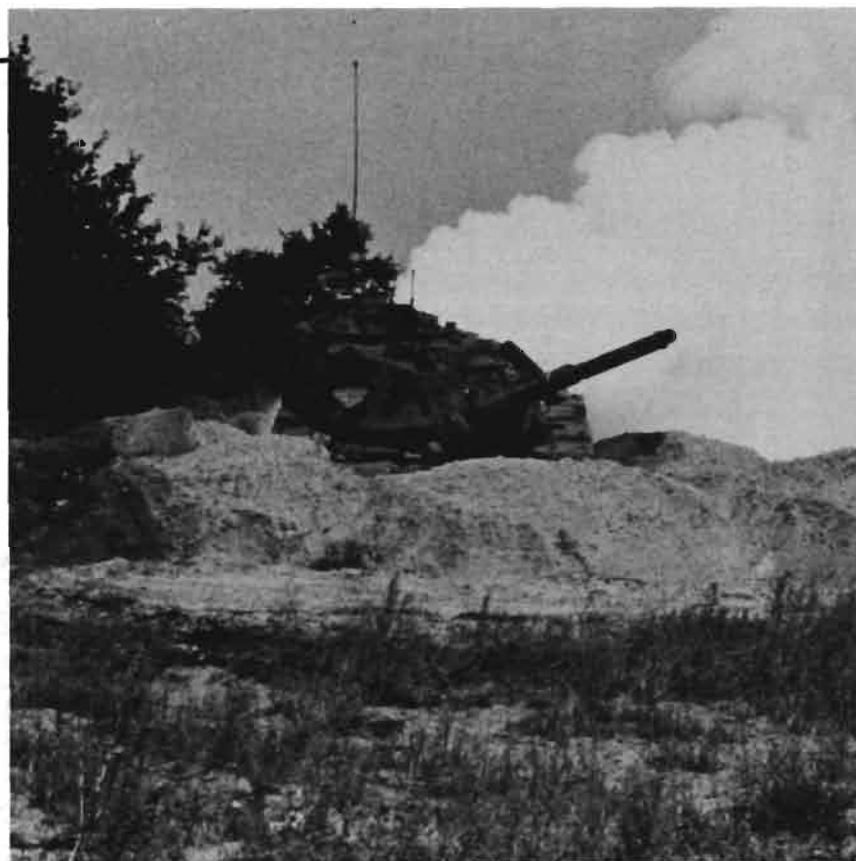
Tank bumps cannot provide defilade for attackers, as tank ditches sometimes can. Loose soil is easily penetrated by modern APFSDS rounds and offers little protection to hull.
