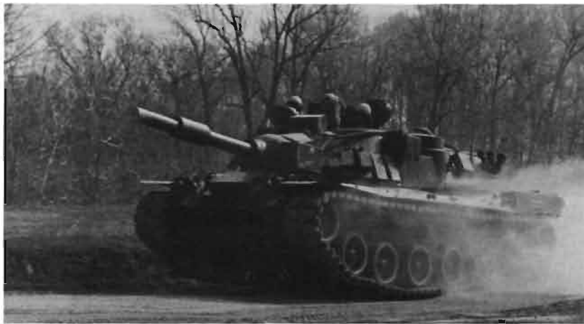
The MBT-70, a joint U.S.-German testbed project, pioneered use of a fin-stabilized kinetic energy round in a gun-launcher system. The gun also fired HEAT rounds and the Shillelagh missile.
