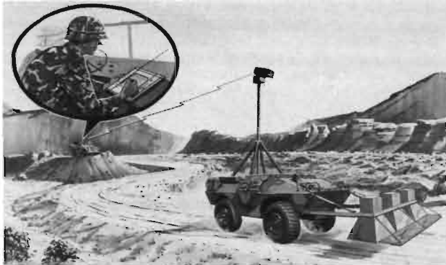
The MIRADOR multi-sensor remotely-controlled minefield reconnaissance and detector system is shown here in an artist's concept sweeping a road for mines and controlled from the jeep in the background.
