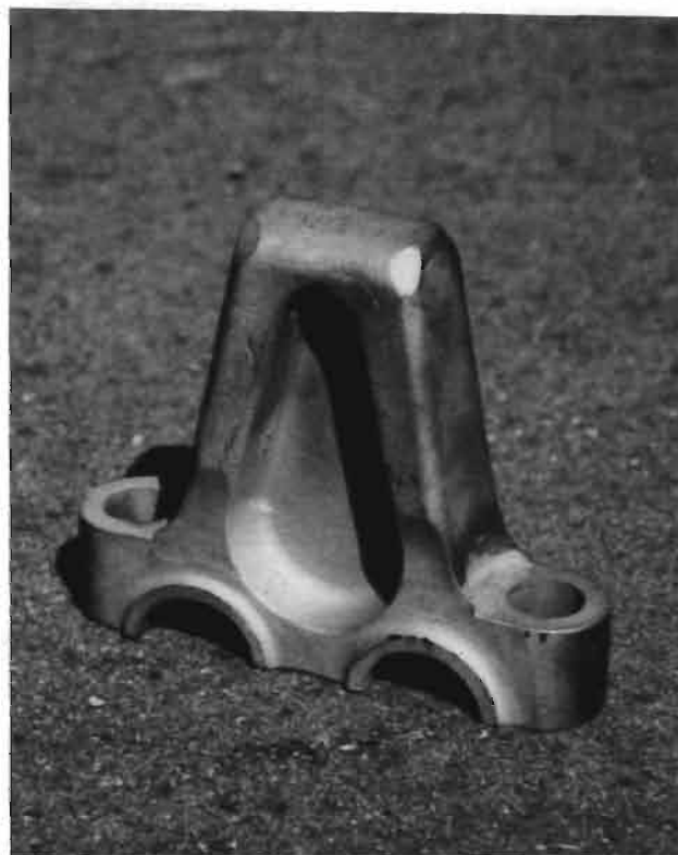
FIGURES 2 AND 3 — New centerguide designs. Figure 2 is simply a lightened form of the centerguide shown in Figure 3.
