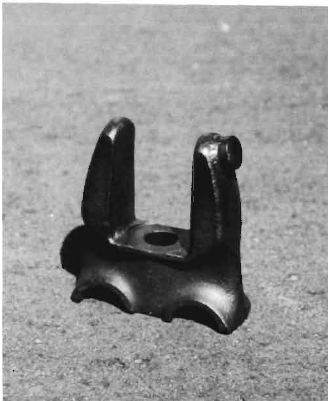
FIGURE 1 — A standard centerguide with a small mass welded on.
