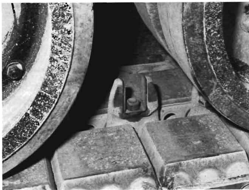
FIGURE 6 — A damper installed on a tank. The dark areas on the centerguide prongs are where the road wheels make contact with the centerguides. These areas will become shiny after a few miles of movement.
