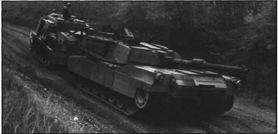
The M88AX tows an M1 at Aberdeen Proving Ground during tests in 1985.
