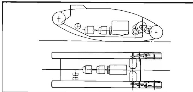
Electric current from a generator, rather than mechanical torque, moves through a cable to electric motors located at each drive sprocket, at a considerable saving in weight and volume. This permits improvements in the general appearance and compactness of the vehicle. Reversing the present circle in armor design permits the following advantages:
