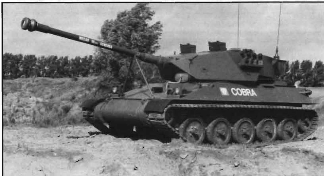
The Cobra 90 light tank, above, and the Cobra 41 APC, at right, are both powered by electric drives, but the powered sprockets are at the rear on the APC and at the front on the Cobra 90. The two vehicles illustrate the flexibility of layout possible with electrical drive. A diesel engine drives the electrical generators in both vehicles.
