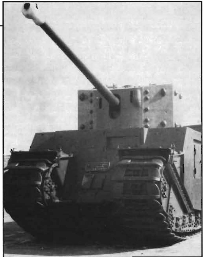
**The TOG, a WWII-era British tank design, used an electrical power transmission system, but was never produced for combat use.**
