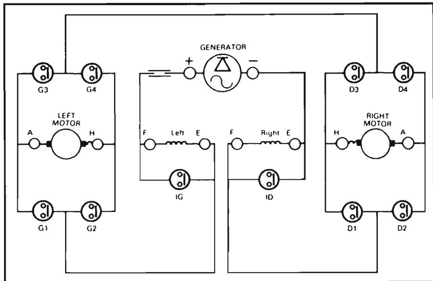
**Electrical schematic of the ACEC drive system for armored vehicles.**
