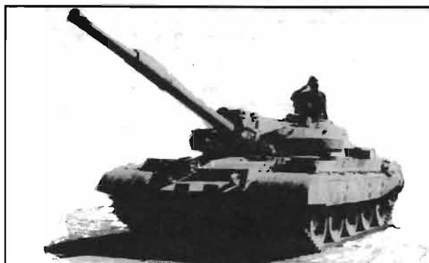
**T-62 modified with applique armor on turret front and sides, non-metallic armor on fuel cells, and rubber side skirts to predetonate HEAT rounds.**
