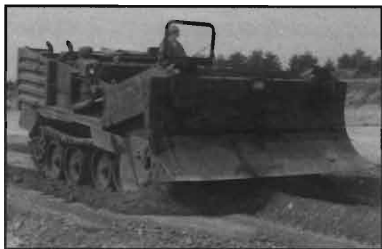
The M9 Armored Combat Earthmover (ACE)
