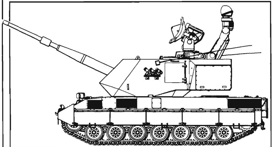
The Navy 76/62 deck gun, with autoloader, is available as a turret unit that can be installed, with its turret basket, in an MBT chassis.
