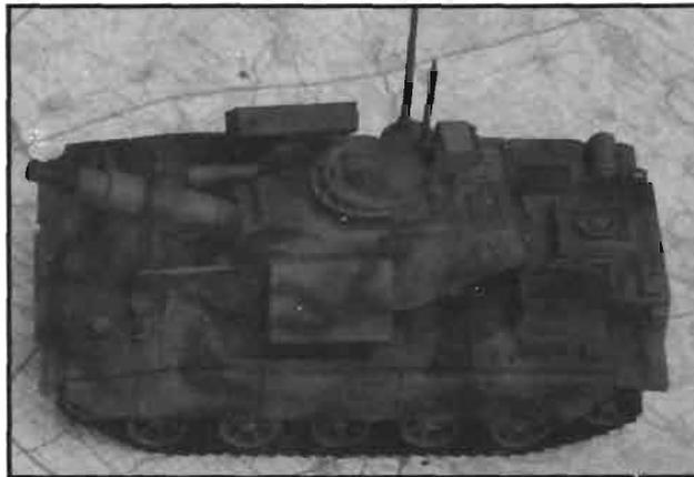
Author-built model includes many of the features he'd like to see in an indirect-fire antitank system, armed with a 120-mm mortar and guided projectiles to engage enemy vehicles from behind cover.
