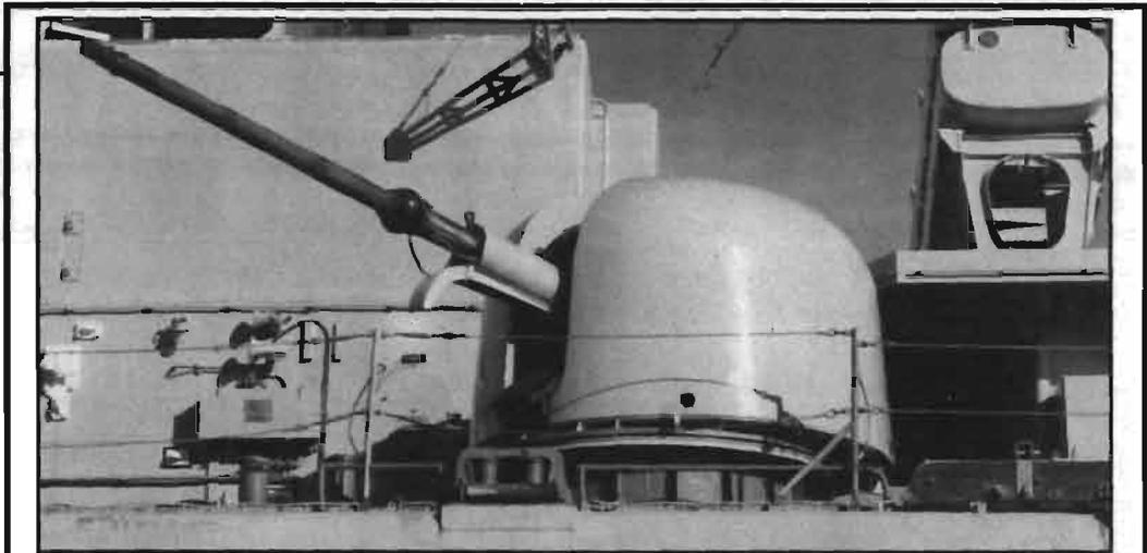
This Italian gun system, widely used as a deck gun by the U.S. and other navies throughout the world, has been adapted to various battle tanks in proof of concept tests by the manufacturer. It is seen here on the deck of the Italian destroyer *Ardito*.
