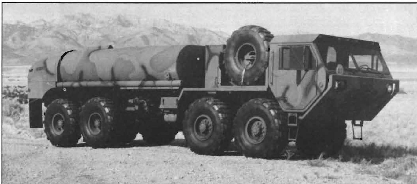
HEMTT fueler's design permits refueling two vehicles at once, on either side.
