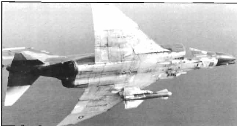
Air Force Phantom with precision-guided GBU-15 under the wing.
