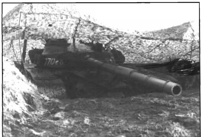
Obscured running gear will reduce Soviet tank thermal signatures.
