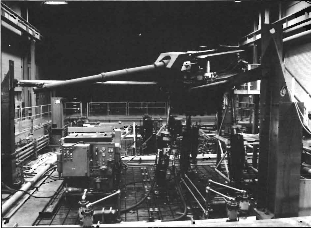
Autoloading turret of the Tank Test Bed Vehicle is suspended in a vibration testing fixture. Rounds stored vertically in the turret basket can be seen below the gun.
