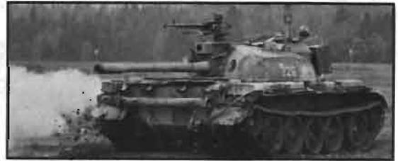
This T-55 is retrofitted with a laser rangefinder.
