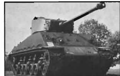
LATE M4A3E8 WITH HVSS SUSPENSION
