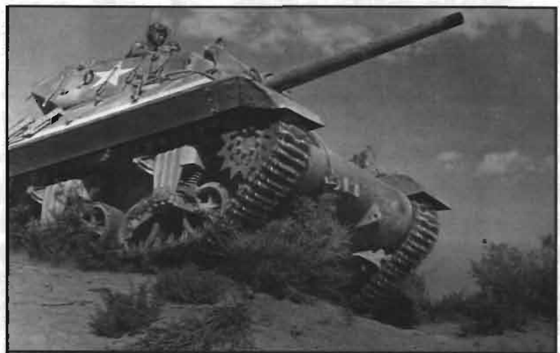
THE M-10 TANK DESTROYER HAD AN OPEN TURRET AND THINNER ARMOR.
