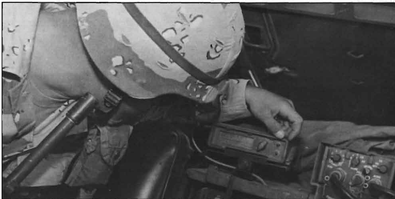
1st Cav trooper checks his position on vehicle-mounted SLGR.
