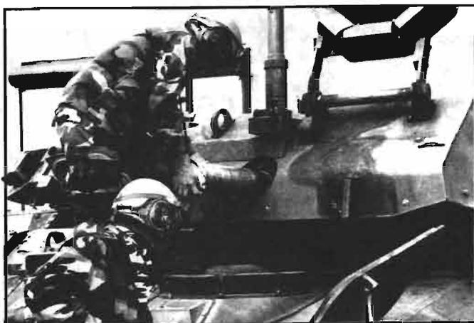
AGS autoloader magazine is replenished through a port in the turret, above. Gunner's computer keeps inventory, indexes proper rounds at gunner's command. At right, the powerpack is on a tray that slides out the rear, allowing quick and easy inspection and repair.
