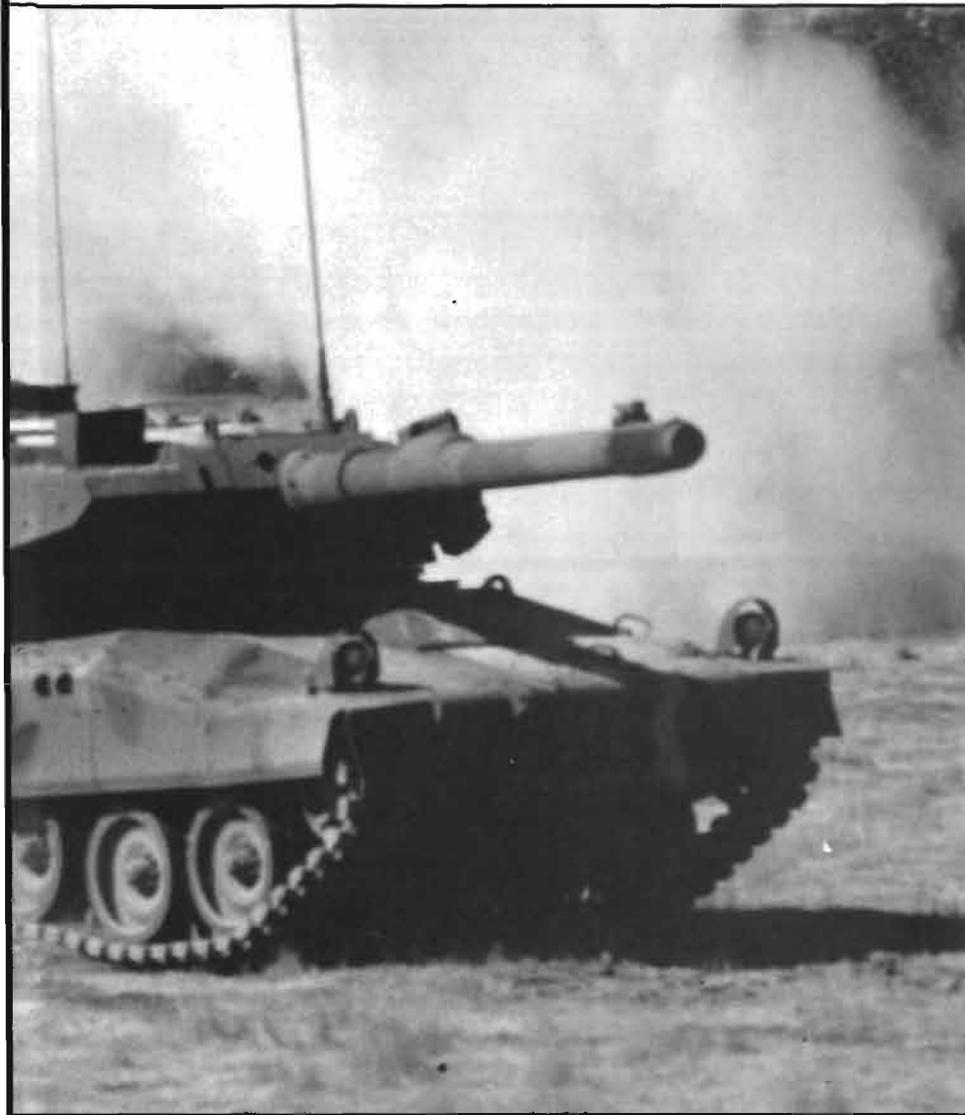
At left, the CCVL prototype that will be the basis for the Army's new Armored Gun System. Because it uses existing components — HEMTT engine, Bradley transmission, LAV 105 primary sight, Challenger 2 fire control computer, etc. — less time will be spent in development
