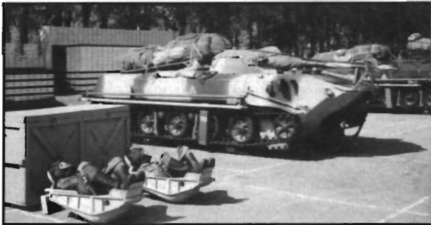
BMD-1, at left, with suspension collapsed and prepared for air drop. Note two soldiers in foreground, mounted in special seats, called "Kintava," that are custom-formed for each man. These two crewmen remain inside the vehicle during the air drop, and the special seats cushion impact. Above right, a BMD variant called the 1V119, similar to a FIST vehicle, is at the center of the static display, with a 2S9 mortar/howitzer version beyond it at far left.
