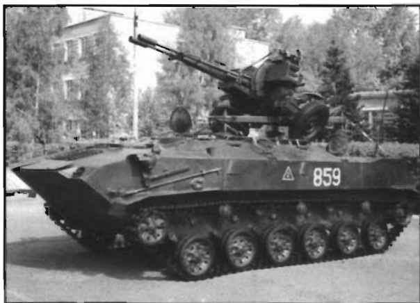
This BMD-2 carries its ZSU-23 twin anti-aircraft gun on the top deck during air drop, then acts as its prime mover once on the ground.
