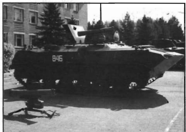
This variant of the BMD is the BTR-RD anti-tank missile vehicle, with launcher on top deck and an additional launcher used in ground mount configuration.
