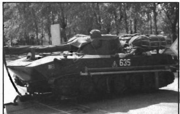
2S9 SP Mortar/Howitzer with suspension collapsed and prepared for air drop. Later BMD variants, like this fire-support vehicle, use longer chassis with six roadwheels, rather than five.
