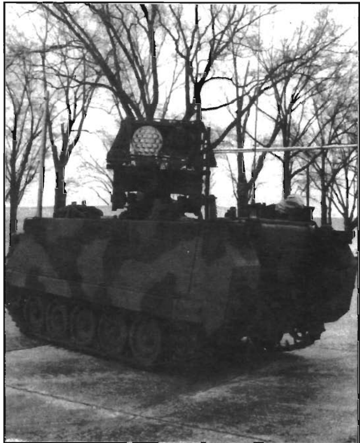
Not a prototype, but a technology demonstrator of a system that will both generate and project smoke from a tracked carrier, the LAMPSS carrier has been exhibited at the Armor Conference, 11th Worldwide Chemical Conference, and at Aberdeen Proving Ground's Armed Forces Day show. It was fabricated in only 45 days at Red River Army Depot, Texas.
