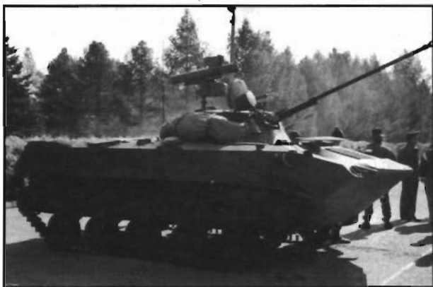
Above, a BMD-2 with 30-mm cannon identical to the 30-mm on the BMP armored personnel carrier. On the turret roof is a launcher mount for the AT-4 missile.
