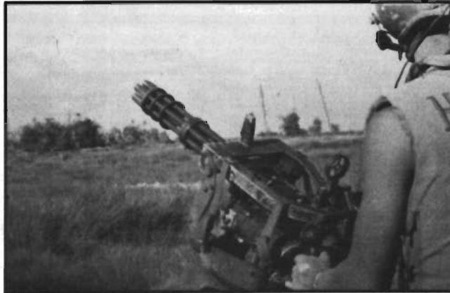
The GAU-2 7.62-mm minigun was one armament option.
