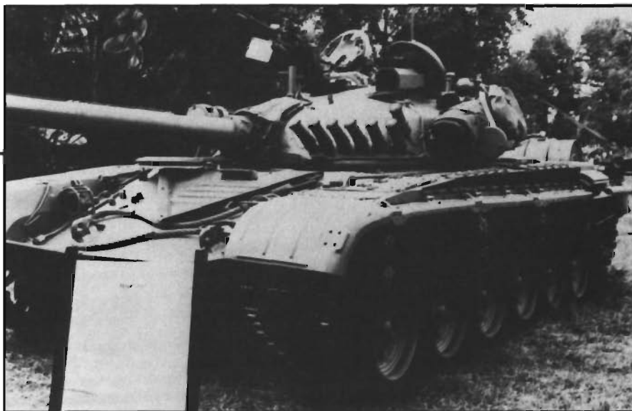
The M-84, a version of the T-72, is manufactured in the former Yugoslavia. This one was part of an order for Kuwait, which purchased the tanks just prior to the Iraqi invasion. Note the non-standard gunner's primary sight and the wind sensor on turret roof.
