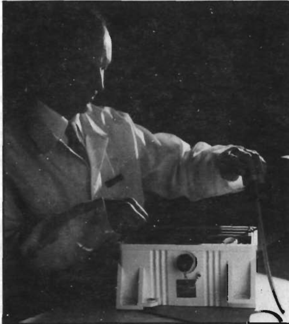
Factory technician makes final adjustments on a POS/NAV navigation system processing unit. Unlike the satellite-dependent Global Positioning System, POS/NAV uses inertial guidance and is self-contained.
