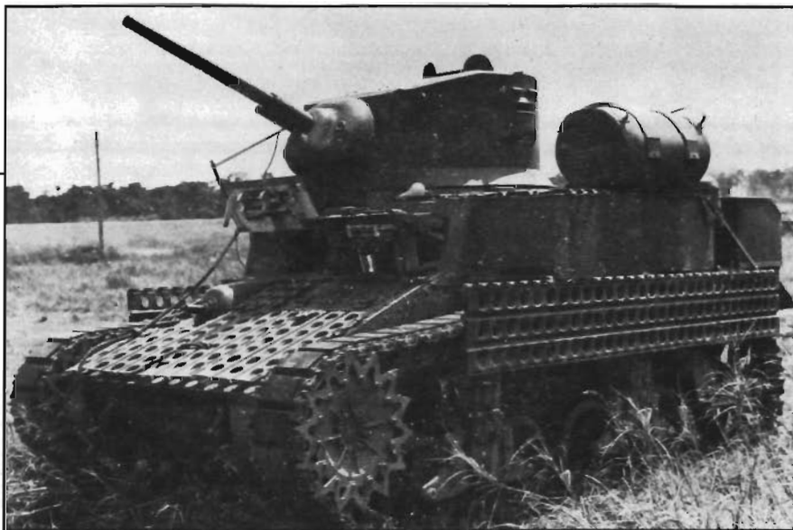
On New Caledonia in 1943, M3A1 light tanks were an earlier attempt to mate flamethrowers with tanks. Their flame nozzles replace the bow machine guns on the right front glacis. Inadequate fuel capacity and poor survivability limited their usefulness. Limited range of the flamethrower can be inferred from bottom photo.
