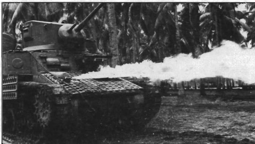
On New Caledonia in 1943, M3A1 light tanks were an earlier attempt to mate flamethrowers with tanks. Their flame nozzles replace the bow machine guns on the right front glacis. Inadequate fuel capacity and poor survivability limited their usefulness. Limited range of the flamethrower can be inferred from bottom photo.
