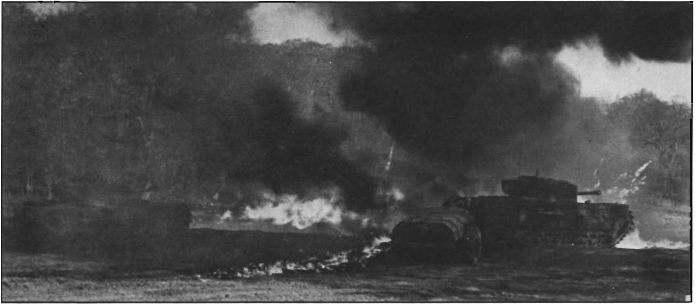
The British Churchill model fitted for flamethrowing was called the "Crocodile." It carried its fuel in an armored trailer and could project a jet of flame over 150 yards. These Crocodiles are seen fighting in France in August 1944.
