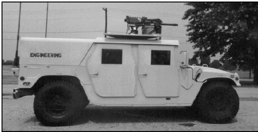
The XM1109, an enhanced armor HMMWV, will protect the crew against shell fragments and 7.62mm armor-piercing rounds fired at 100 meters or more. Windshields and side windows are armored. Shown here with the Scout Platoon Modification Kit, this vehicle is armed with the Mk 19 grenade launcher and fitted with a TOW sight (AN/UAS-11 or AN/UAS 12), GPS, and 2-radio SINCGARS capability, along with a 100-amp alternator.
