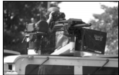
The XM1109, an enhanced armor HMMWV, will protect the crew against shell fragments and 7.62mm armor-piercing rounds fired at 100 meters or more. Windshields and side windows are armored. Shown here with the Scout Platoon Modification Kit, this vehicle is armed with the Mk 19 grenade launcher and fitted with a TOW sight (AN/UAS-11 or AN/UAS 12), GPS, and 2-radio SINCGARS capability, along with a 100-amp alternator.
