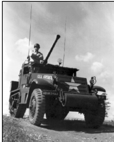
Halftracks soldiered on after the war and saw action in Korea. Some were employed as troop carriers; others carried mortars or anti-aircraft guns. This one mounts a 40-mm AA gun.
