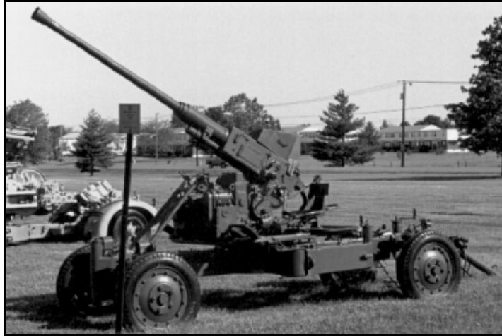
Figure 7. The 40mm L/60 Bofors anti-aircraft gun, a 1936 design, saw wide use in many countries. This one, displayed at Aberdeen Proving Ground, is a U.S. Army M1A1 version of the WWII era. (Author's Photo)
