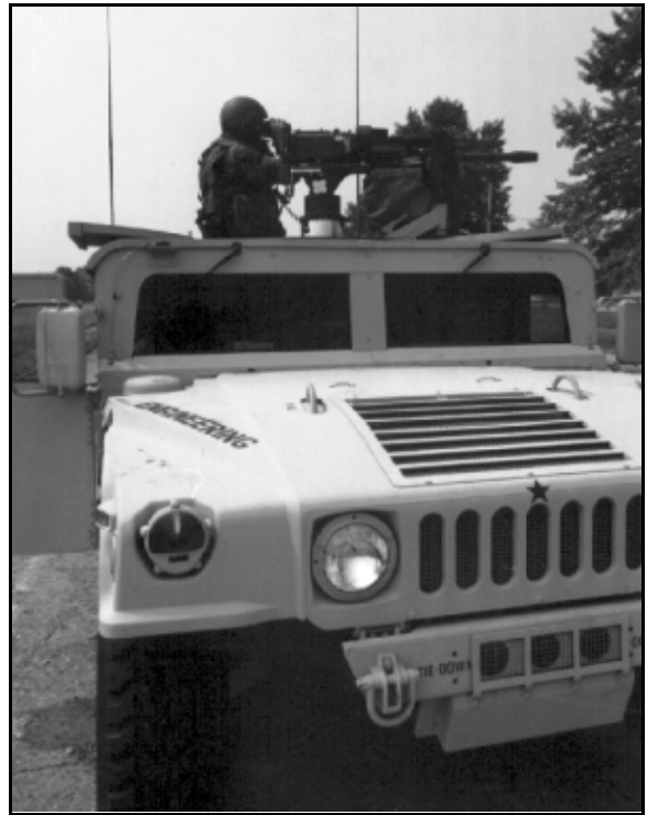
The M1109 HMMWV, with the Scout Platoon Modification Kit, was displayed recently at Fort Knox. It includes better protection for the crew from mines, bullets, and shell fragments, improved observation and navigation equipment, and greater carrying capacity for scout stowage.
