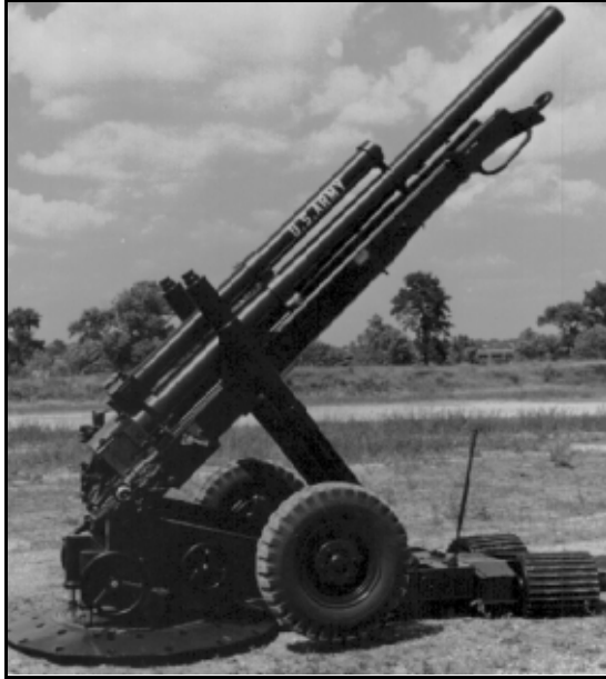
Figure 1. The U.S. M204 105mm howitzer, developed in the mid-'70s, employed the differential recoil principle, but never went into production.
