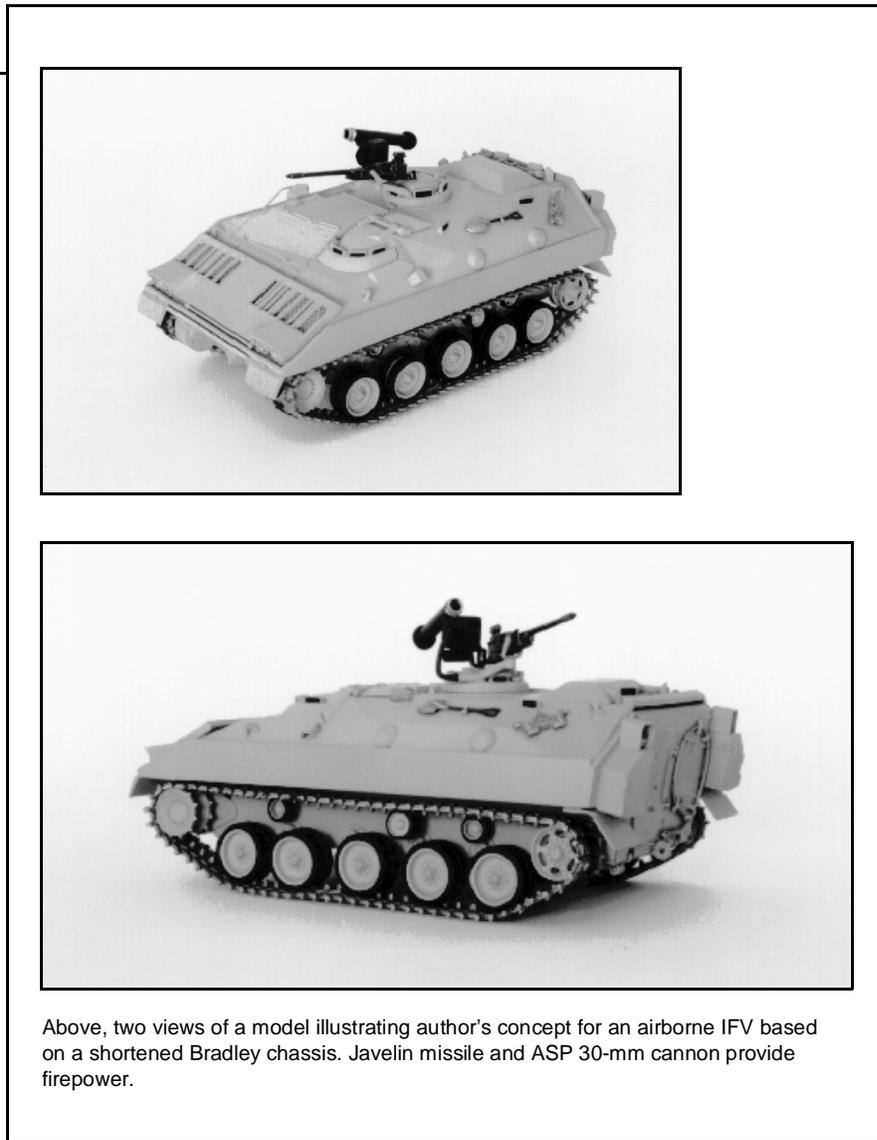
Above, two views of a model illustrating author's concept for an airborne IFV based on a shortened Bradley chassis. Javelin missile and ASP 30-mm cannon provide firepower.
