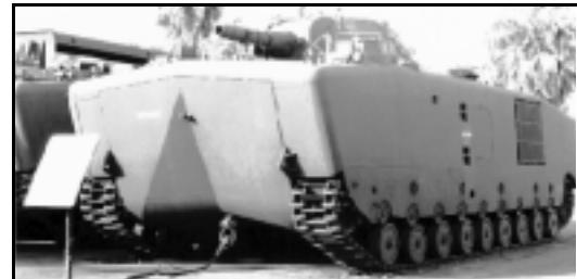
105-mm howitzer, which was originally armed with a 75-mm gun; and the LVT(A)4 amphibian tractor with 75-mm howitzer, which was originally armed with a 37-mm gun. Both of these vehicles were extensively and successfully used in combat.
