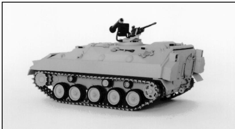
Above, two views of a model illustrating author's concept for an airborne IFV based on a shortened Bradley chassis. Javelin missile and ASP 30-mm cannon provide firepower.
