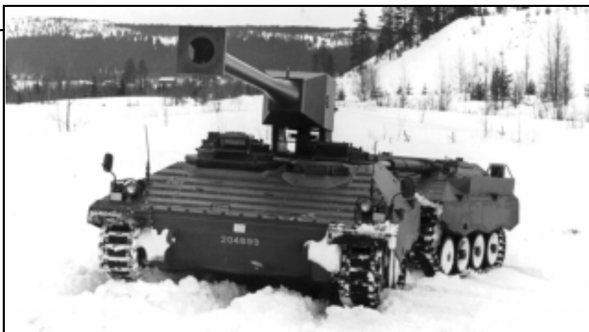
Two Swedish concept vehicles, the UDES-19, at left, seen in model form, and the articulated UDES-20, above, were external gun designs. The arm seen at the base of the UDES-19's gun pedestal was the device used to transfer ammunition from the hull to the rear of the gun.
