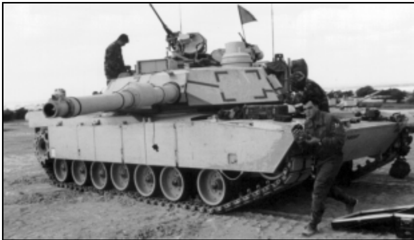
At left, a crew installs the TWGSS system to an M1A2 at Fort Hood. It takes 20 minutes. Above, a crew reviews the after-action record that is stored on a laptop computer.
