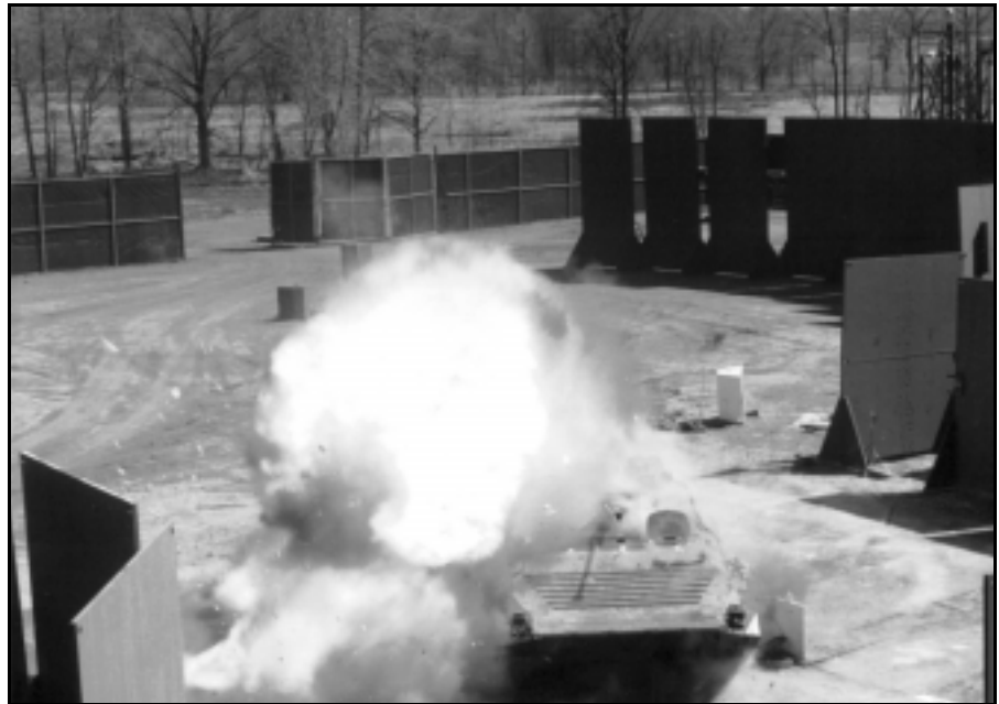
The BMP at moment of Javelin warhead ignition. Note armor plate shields around test area to ensure safety.
