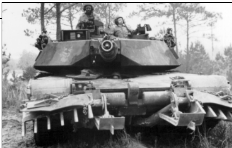
Here, the TWGSS system is mounted on a Marine M1A1 at Camp Lejeune, N.C. The Marines use the system for both tactical and gunnery training.
