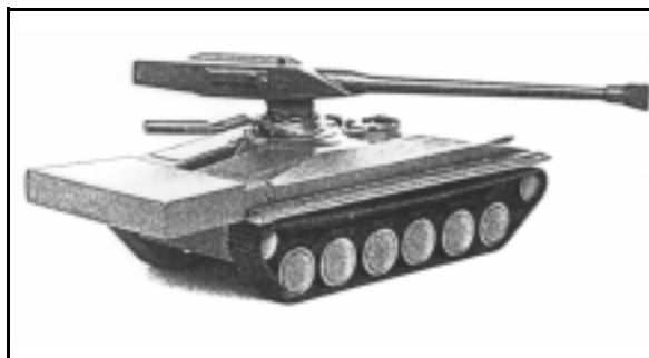
Two Swedish concept vehicles, the UDES-19, at left, seen in model form, and the articulated UDES-20, above, were external gun designs. The arm seen at the base of the UDES-19's gun pedestal was the device used to transfer ammunition from the hull to the rear of the gun.
