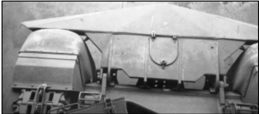
TOP VIEW: Hollow blade is angled to push brush aside.
