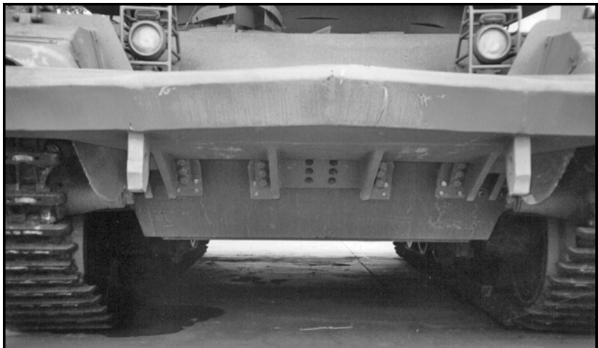
FRONT VIEW: Blade mounted on front slope shows anchoring points
