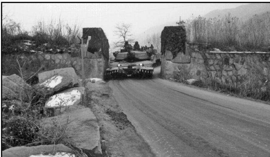
M1A1 passes through a “rock-drop” point obstacle on a division 2-way supply route.
