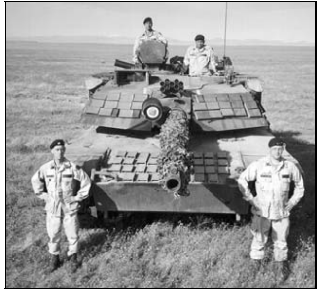
Nevada Army National Guard soldiers in their OPFOR uniforms show off an M1 tank they modified to look like a T-80. The M1's skirts were removed, "reactive armor" blocks were added, along with drum-like auxiliary fuel tanks, a searchlight, and a snorkel tube at rear of turret.
