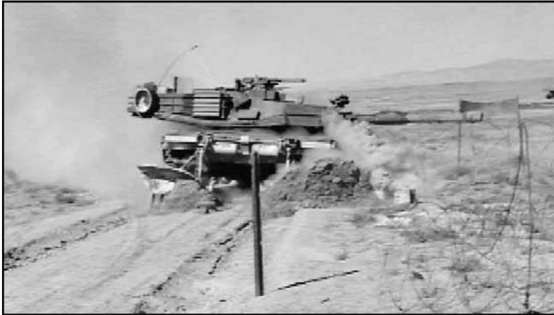
Mine plow-equipped M1A1 rolls down the lane at Gowen Field.
