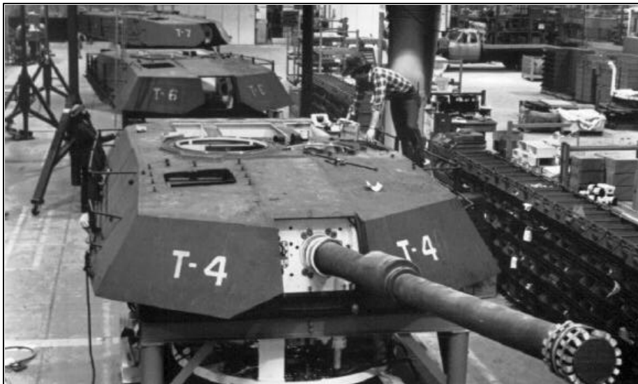
Early production M1 turrets move down the Chrysler production line.
