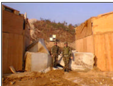
Photo sequence shows effect of the new round on a typical Korean "rock drop" obstacle, seen intact at upper left. Obstacle blocks have dropped in lower left photo which shows size of the blocks compared to standing soldiers. Above, the rubble left after demolition by the new XM908 round.
