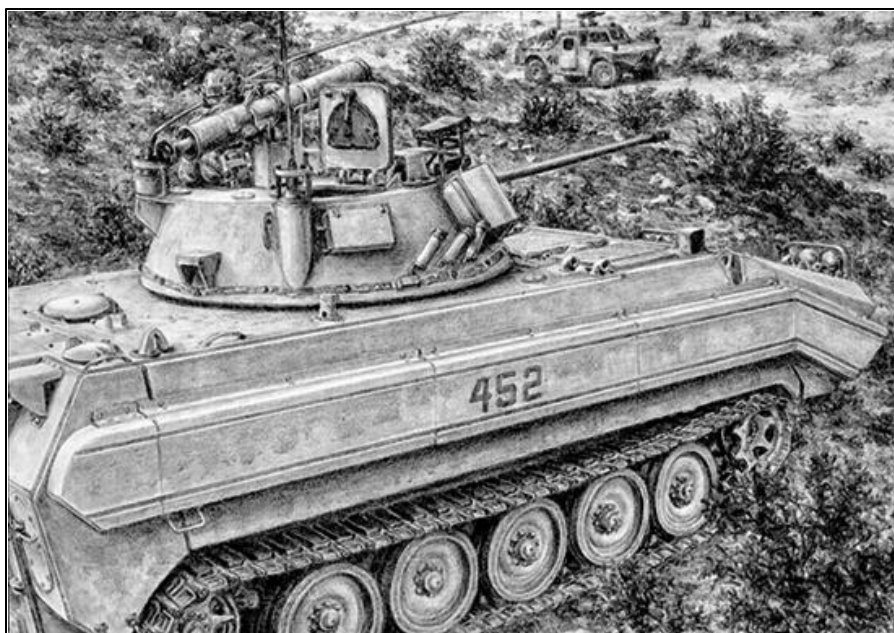
The OPFOR Surrogate Vehicle (OSV), based on the M113 APC with visual modifications that make it resemble a BMP, will expand tactical capabilities by allowing dismounts to be carried. —Jody Harmon Sketch
