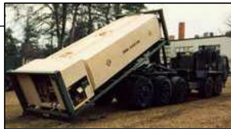
Fuel tank and pump unit.
