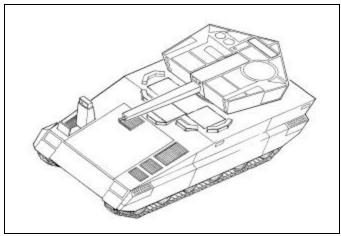
Conceptual vehicle is seen above in travel mode, and at right insurveillance mode with sensor systems deployed. Main gun tube housing also contains antenna array and is raised to vertical when sensors are deployed.
