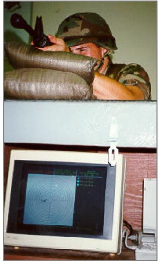
The results of SGT Megow's three-round shot group. The darker circle on the monitor indicates the center of mass of the three-round group. The results are within the 40mm dispersal required.
