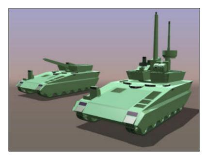
emy. Stringent operational requirements have been posted for a small and light vehicle featuring a low profile, increased agility, and improved mobility to enhance its survivability. These requirements led to various vehicle configurations that were inadequately protected — if at all — thereby suffering a highly disproportional casualty rate when exposed to hostile enemy fire.
