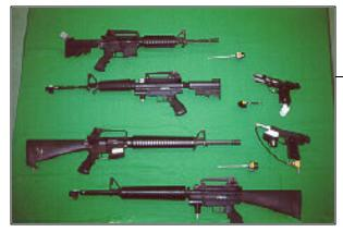
The pneumatic weapon replicas. From top to bottom, left to right, an M4 carbine, a laser transmitter and rod for the M4/M16A2, a pneumatic M4, an M9, a laser transmitter and rod for an M9, a pneumatic attachment for a .45 cal pistol (now available for an M9), an M16A2, a laser transmitter and rod for the M4 / M16A2, and a pneumatic M16A2.
