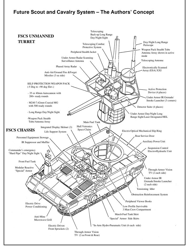
To ensure that the FSCS will survive to achieve its entire mission and ultimately return safely, it must be equipped with state-of-the-art *defensive* protection and weapon systems. These will dramatically enhance its survivability and provide independence from reliance on the forces it is designated to support, allowing it to independently operate close to enemy front lines.
