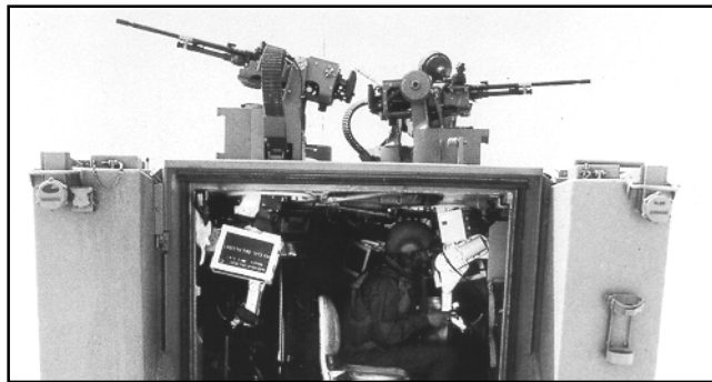
Top, overhead weapon station (OWS) assemblies mount 7.62mm machine guns above day/night sight unit and internal controls. Flexible chute feeds ammunition from 230-round box. Above, an internal view of an M113 with overhead weapon stations installed. Single gun unit is at right. OWS machine guns can be also fired from the open hatch, as shown in top photo. (Photos: Rafael, Israel)
